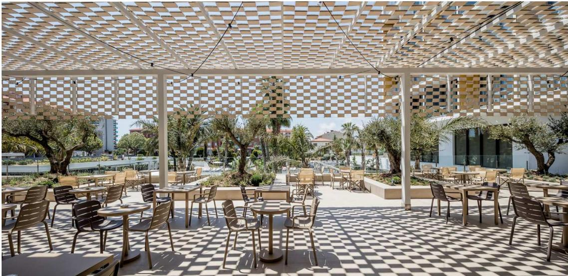
*Technical details. Square meters installed: 675 - Number of sheets: 93 - Size of the ceramic tile: 20 x 10 x 3 cm - Fretwork: 42-50% - Material of the ceramic tiles: single-color terracotta - Mesh and support of the façade: AISI 316 stainless steel - Mean length of sheets: 6 meters - Construction time: 12 days - Architecture firm: Isern Arquitectos.*
